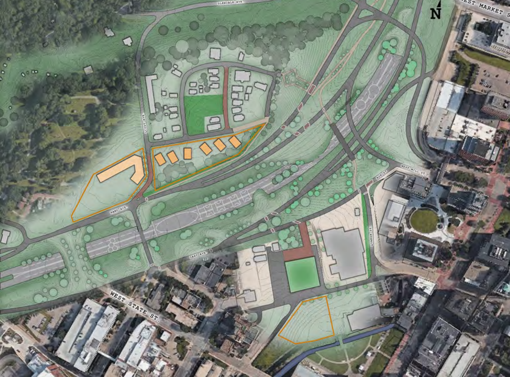
Above: Site plan showing the final potential buildout on either side of the Innerbelt trench, including a new State St land bridge and a reconnected Locust St.
